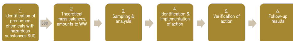
Figure 7. Six steps of process mapping of hazardous substances
