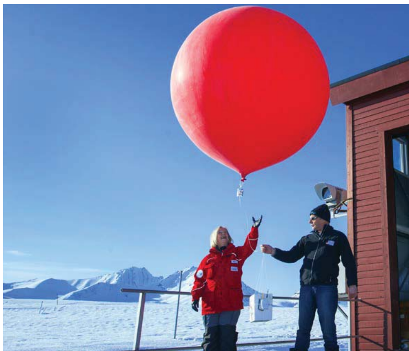
Sending up measuring instruments attached to a balloon enables important information to be obtained about the vertical distribution of the ozone layer in the atmosphere.
