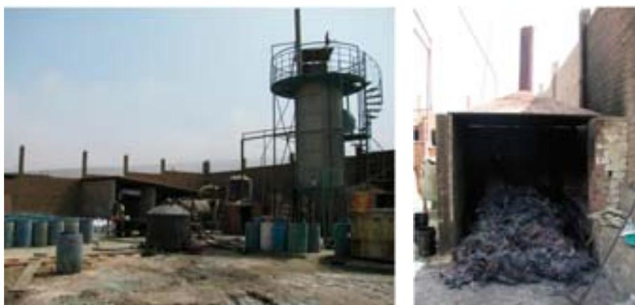
Figure 26. Simple facility for recycling of copper cables, showing the whole facility to the left and the cable burning furnace to the right. Ash sample 1 was collected here (Photos: © Viktor Sjöblom).
