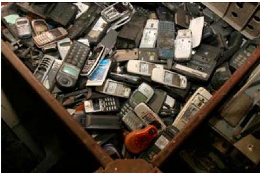
Figure 4. E-waste, such as these obsolete mobile phones, contains a variety of materials including plastics, metals, and glass (Photo: © Juraj Rizman, Greenpeace).
