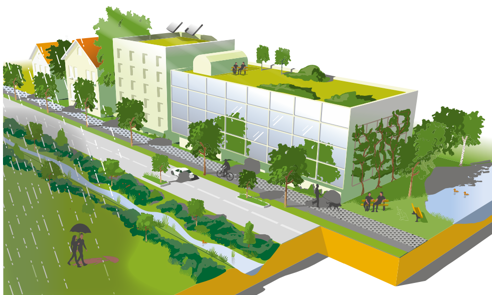
Figure 11. Examples of nature-based solutions in urban environments: green roofs, urban greenery, urban trees, rain gardens, swales, stormwater ponds and permeable surfaces.
