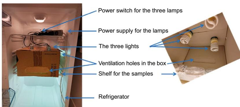
Figure 3. The homebuilt UV-B treatment facility. The lamps were installed in a cardboard box. Two ventilation holes was cut into the cardboard box sides. The box were placed on a shelf in a refrigerator on maximal cooling, about the lamps were placed approximately 10–15 cm from the shelf where the samples were placed.
