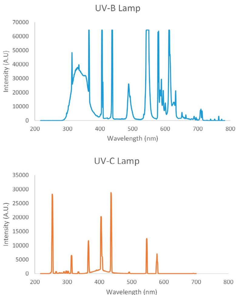
Figure 1. Spectrum for the UV-B, upper panel, and UV-C lamps, lower panel.
