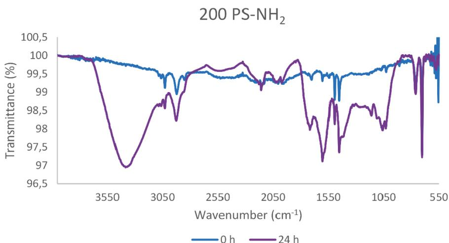
Figure 4. The figure shows the surface chemistry, determined with ATR-FTIR, on 200 nm aminated polystyrene particles before, in blue, and after, in purple, 24 hours UV-C treatment.
