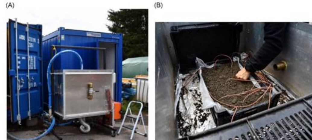
Figure 1. (A) Steaming rig and (B) container of prototype device used in the experiments. Photos: Belachew Asalf Tadesse.
