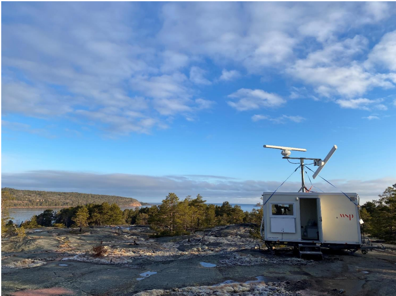
Figure 2. Setup of bird radar station at Dånö, Langnäs on the northern side of Åland. The setup is complete with a horizontal and vertical radar mounted on top of a trailer-wagon. The horizontal radar is used to determine the flight direction of migrating birds, while the vertical radar is used to determine flight height and migration intensity.
