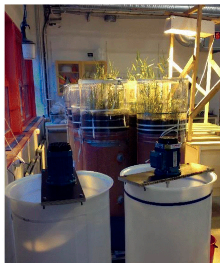
Figure B8. Bioretention column design used in laboratory testing by Søberg et al. (2020). Published under Creative Commons Attribution (CC BY 4.0) license.
