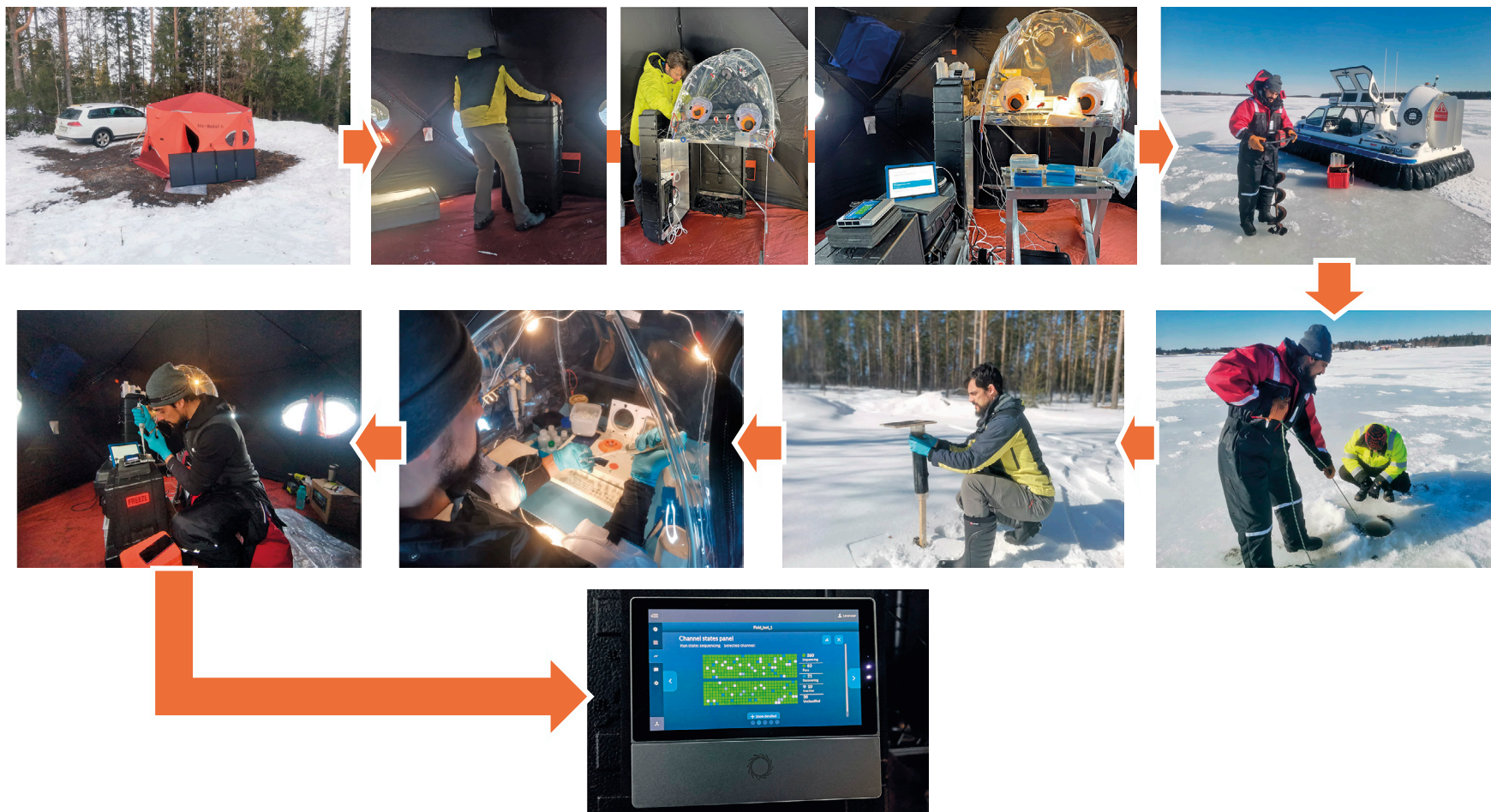
Figure 3. Field experiment carried out to test OmiBox performance in the field under cold conditions, from OmiBox deployment to sample collection, processing and sequencing.
