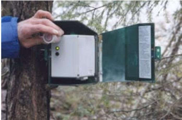
Battery power is sufficient and the settings are functional when the red indicator lamp does not light up.
