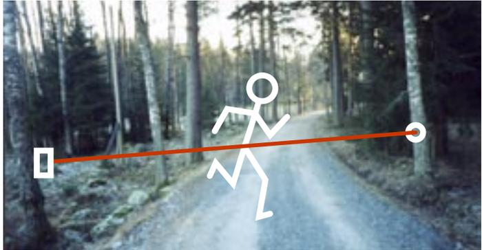
Passersby are recorded when the beam of infrared light between the counter and the reflector is interrupted.
