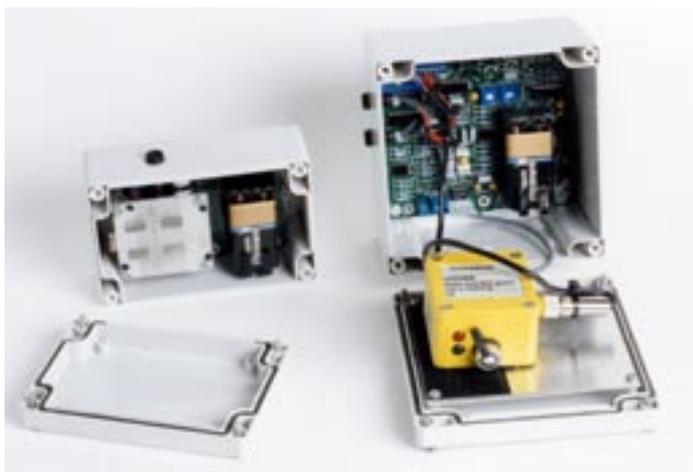
Transmitter and receiver with logger connected.
