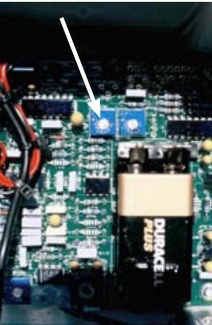
With the RV2 function, the transmitter's signal pulse can be adjusted, for example to exclude horseback riders from the count.
